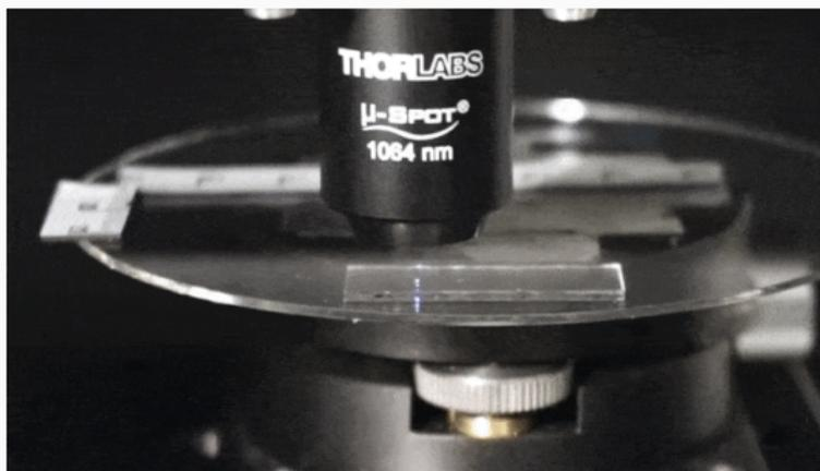
By focusing a femtosecond laser beam on silica glass we slightly modify the local refractive index, inducing waveguiding [2].
